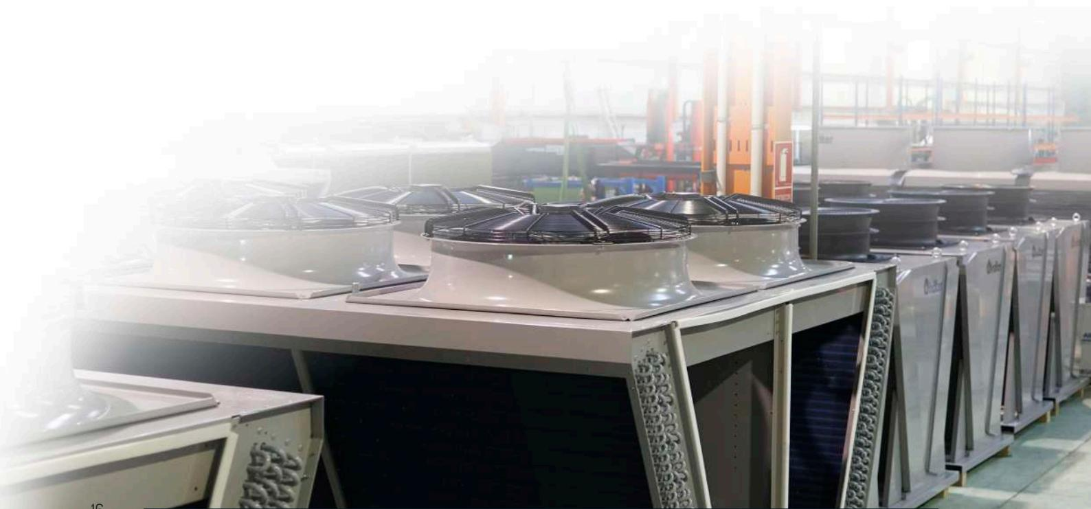
ATMF series corresponds to the air coolers/heaters portfolio for air conditioning purposes working both on cooling or heating mode with single-phase and three-phase fans, for the standard version, which cover a range of capacities from 11 kW up to 35 kW for cooling mode and from 13 up to 42 kW for heating mode.
